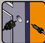
DRILL DOOR HOLES
